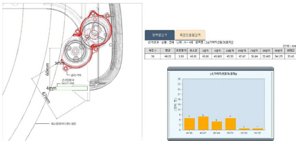
Figure 4. Roller position after due consideration about child's finger
